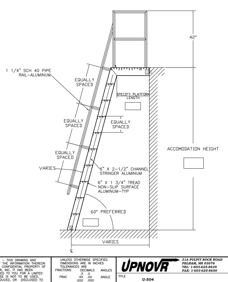
NOTICE — THIS DRAWING AND ALL OF THE INFORMATION THEREON IS THE CONFIDENTIAL PROPERTY OF UPNOVR, INC. IT HAS BEEN PROVIDED TO YOU FOR A LIMITED PURPOSE IS NOT TO BE USED, REPRODUCED, OR DISCLOSED TO OTHERS FOR ANY OTHER PURPOSE. ALUMINUM SHIP'S LADDER WITH **APPROVALS** DATE **PLATFORM** MATERIAL DRAFTED ALUMINUM SIZE PART/PROJ. No. DWG. NO. REV. U-504 В CHECKED Α **TREATMENT APPROVED** NTS QTY REQ'D SHEET SCALE
